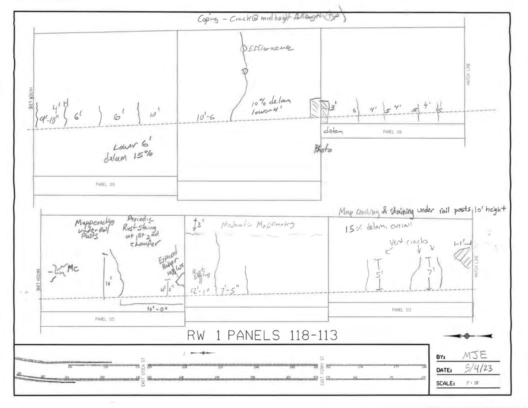
119 has light can televood from face 383 cores /delan delam chamfer lowers Crack Rebar lower 41 is 50% spalled & delan Exposel Cracks every 21 Stain Photo 2 Photo PANEL 119 PANEL 121 RW 1 PANELS 121-119 MJE BY: 5/4/23 DATE: SCALE: 1" = 10'
